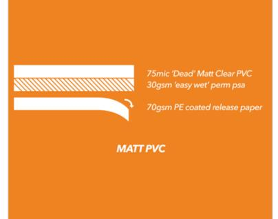
Matt clear PVC is a 'dead' matt clear PVC overlaminating film which is coated with a permanent acrylic adhesive suitable for overlamination of all ink types including UV inks. The 'dead' matt smooth finish gives absolutely excellent anti-glare properties and therefore this product is commonly used for general paper and filmic poster graphic overlamination where a matt clear completely anti-glare or 'dead' matt finish is required.
